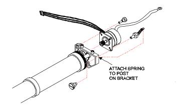
Figure 5-15. Stepper Motor Removal/Installation.
